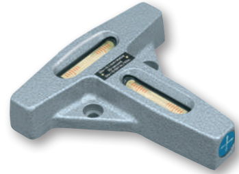
Model C: T-shaped level with cross vials, 2-point mounting. Manually lapped measuring base to ensure a much higher precision of the level.
