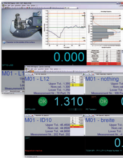
Measuring display with the option of adding operational instructions, accompanied with a photo or drawing
